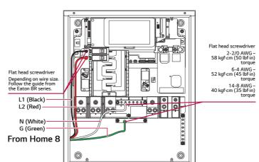
11 Insert the communication wires into the 6-position connectors.
