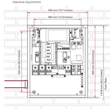
**2** Fix the SE Box with 4EA screws and anchors with 0-rings in each position. Before fastening the screws, place the supplied 0-rings on the screws.
