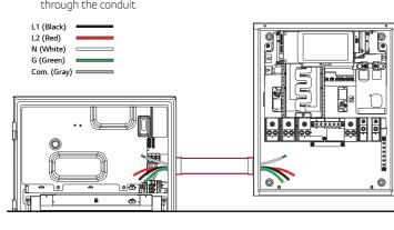
3 Strip off the AC power conductors (L1, L2, Neutral, and Ground) on both the Home 8 and SE Box sides as shown in the figure below.
