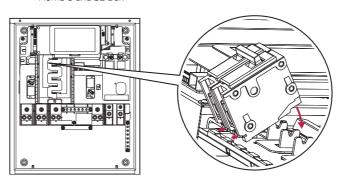
[10] connect the AC conductors to the corresponding terminals
