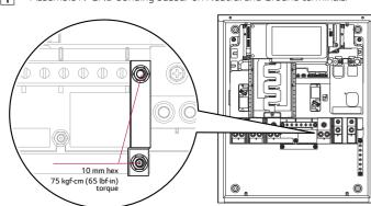
Install a compatible main breaker by fastening the 2 nuts.
