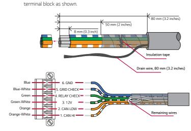
6 On the SE Box side, strip the 6-conductor communication cable as shown in the figure.
