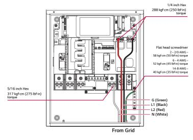
2 Connect the home load conductors (L1, L2, Neutral, and Ground) to the SE
