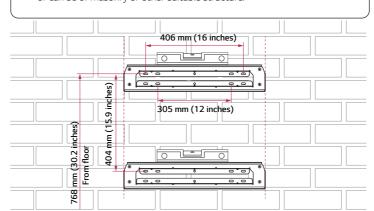
Affix the wall bracket to the wall with screws or anchors.
