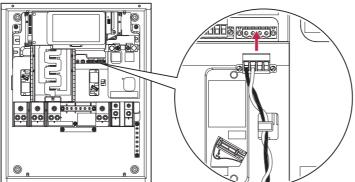
5 Arrange the power cables and fasten them using a cable tie.
