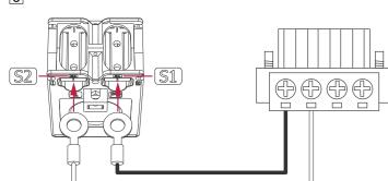
Pass the PV L1 cable from the PV inverter through the 200 A CT  $\,$
